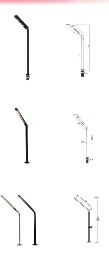
Model:Stalk PAR120A Wattage:3W Voltage:AC110-240V Current:300mA LED Source:Osram LED CCT:2700-6000k Lumen:330-390lm CRI:Ra80/93 Beam angle:25/45° IP:IP20 Material:Aluminum Shell colour:Anodised silver/black/gold Cut size:Ф12mm
