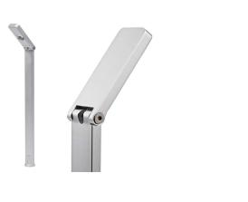
Model:Stalk PAR122E Wattage:4W Voltage:AC110-240V Current:300mA Height:Custom made LED Source:Cree COB CCT:2700-5000k Lumen:400lm CRI:Ra80/93 Beam angle:60° IP:IP20 Material:Aluminum Shell colour:Anodised silver/black Cut size:Ф10mm
