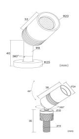
Model:Surface Mount PAR101-1 Wattage:2W Head rotary:360° Voltage:DC12V/AC110-240V Current:500mA LED Source:Osram LED CCT:2700-6000k Lumen:120-180lm CRI:Ra80/93 Beam angle:10/30/60° IP:IP20 Material:Aluminum Shell colour:Anodised silver/black/gold Installation:Screw fix or surface mounted
