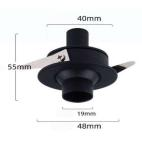
Model:Recessed PAR108-10 Wattage:3W Dimension:Ф48\*55mm Cut size:Ф40mm Voltage:AC110-240V Current:350mA LED Source:Osram LED CCT:2700-6000k Lumen:80-100lm CRI:Ra80/93 Beam angle:5/15/25/45 IP:IP20 Material:Aluminum Shell colour:Anodised silver/black/gold Installation:Recessed
