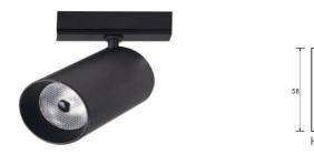
Model:Micro-Line Trak 10-04 Wattage:5W Head rotary:355° Voltage: DC12-24V Non-dimmable DC24V Dimmable CCT:3000K/4000K/6000K Lumen:450lm SDCM<3 CRI:Ra95 Beam angle:5/15/25/45° IP:IP20 Dimmable:PWM/0-10V/Dali Material:Aluminum Shell colour:Anodised silver/black
