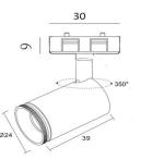
Model: Mini-Trak 115-2 Wattage:3W Head rotary:355° Voltage:DC12V/DC24V Non-dimmable LED Source:Osram LED CCT:2700-6000k Lumen:175Im CRI:Ra80/93 Beam angle:10-60° IP:IP20 Material:Aluminum Shell colour:Anodised silver/black
