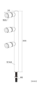
Model:Stalk PAR112B Wattage:2-10W Height:Custom made Voltage:AC110-240V Current:300mA LED Source:Osram LED CCT:2700-6000k Lumen:120lm/Head CRI:Ra80/93 Beam angle:25/45° IP:IP20 Material:Aluminum Shell colour:Anodised silver/black/gold Cut size:Ф8mm
