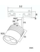
Model: Mini Trak 103-2 Wattage:3W Head rotary:355° Voltage:DC12V/DC24V Non-dimmable Current:250mA LED Source:Osram LED CCT:2700-6000k Lumen:200-300lm CRI:Ra80/93 Beam angle:15/30/60° IP:IP20 Material:Aluminum Shell colour:Anodised silver/black
