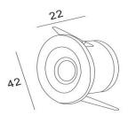
Model:Recessed PAR108-3 Wattage:2W Dimension:Ф42\*25mm Cut size:Ф36mm Voltage:AC110-240V Current:350mA LED Source:Osram LED CCT:2700-6000k Lumen:200lm CRI:Ra80/93 Beam angle:45° IP:IP20 Material:Aluminum Shell colour:White/black Installation:Recessed
