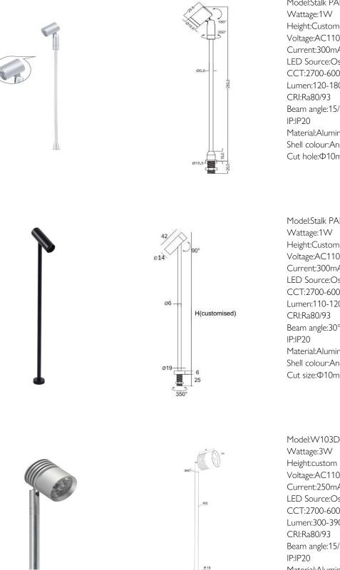
Model:Stalk PAR102 Wattage:1W Height:Custom made Voltage:AC110-240V Current:300mA LED Source:Osram LED CCT:2700-6000k Lumen:120-180lm CRI:Ra80/93 Beam angle:15/40° IP:IP20 Material:Aluminum Shell colour:Anodised silver/black/chrome Cut hole:Ф10mm
