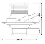
Wattage:5W Dimension:  $\Phi74*70$ mm Cut size:064mm Voltage:AC110-240V Current:700mA LED Source:Osram LED CCT:2700-6000k Lumen:300-380lm CRI:Ra80 Beam angle:10-60° zoomable IP:IP20 Material:Aluminum Shell colour: Anodised silver/black Installation:Recessed
