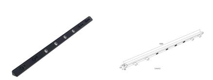
Model: Linear Spot 532-V Wattage:8W Voltage:DC24V/AC110-240V Dimension:500mm LED Source:Osram LED CCT:2700-6000k Lumen:100lm/Head CRI:Ra80/93 Beam angle:25/45/60° IP:IP20 Material:Aluminum Shell colour:Anodised silver/black/gold Installation:Screw fix/surface mounted
