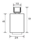
Model:Micro-Line Trak 10-06 Wattage:3W Head rotary:355° Voltage: DC12-24V non-dimmable DC24V Dimmable CCT:3000K/4000K/6000K Lumen:250lm SDCM<3 CRI:Ra95 Beam angle:5-60° IP:IP20 Dimmable:PVM/0-10V/Dali Material:Aluminum Shell colour:Anodised silver/black
