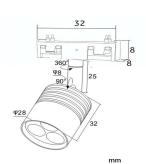
Model: Mini Trak 103-2 Wattage:3W Head rotary:355° Voltage:DC12V/DC24V Non-dimmable Current:250mA LED Source:Osram LED CCT:2700-6000k Lumen:200-300lm CRI:Ra80/93 Beam angle:15/30/60° IP:IP20 Material:Aluminum
