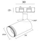
Model: Mini-Trak 115-2 Wattage:3W Head rotary:355° Voltage:DC12V/DC24V Non-dimmable LED Source:Osram LED CCT:2700-6000k Lumen:175lm CRI:Ra80/93 Beam angle:10-60° IP:IP20 Material:Aluminum Shell colour:Anodised silver/black
