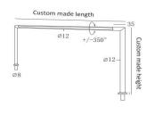
Model:Bridge 019 Wattage:16W/Meter Profile size:Φ12mm Voltage:DC12V Height:Custom Made LED Source:210PCS SMD CCT:3000-6000k Lumen:100lm/Watt CRI:Ra80/93 Beam angle:60° IP:IP20
