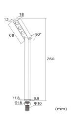
Model:Stalk PAR122B Wattage: 3W/5W Voltage:AC110-240V Current:300mA Height:Custom made LED Source:Osram LED CCT:2700-6000k Lumen:120lm/W CRI:Ra80/93 Beam angle: 25/45/60 IP:IP20 Material:Aluminum
