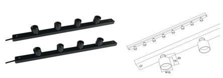
Model:Linear Spot 533-U Wattage: 2W-20W Aluminum profile:11\*11mm Voltage:DC24V/AC110-240V Length:150-2000mm LED Source:Osram LED CCT:2700-6000k Lumen:100lm/Head CRI:Ra80/93 Beam angle:25/45/60° IP:IP20 Material:Aluminum
