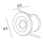
Model:Recessed PAR108-3 Wattage: 2W Dimension:Φ42\*25mm Cut size:Φ36mm Voltage:AC110-240V Current:350mA LED Source:Osram LED CCT:2700-6000k Lumen:200lm CRI:Ra80/93 Beam angle:45° IP:IP20 Material:Aluminum Shell colour:White/black
