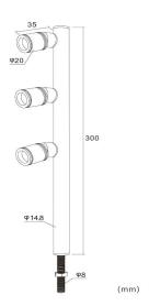
Model:Stalk PAR112B Wattage:2-10W Height:Custom made Voltage:AC110-240V Current:300mA LED Source:Osram LED CCT:2700-6000k Lumen:120lm/Head CRI:Ra80/93 Beam angle:25/45° IP:IP20 Material:Aluminum Shell colour: Anodised silver/black/gold
