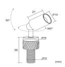
Model:Surface Mount PAR111-1 Wattage:1W Height:Custom made Voltage:DC12V/24V/AC110-240V Current:300mA LED Source:Osram LED CCT:2700-6000k Lumen:80lm CRI:Ra80/93
