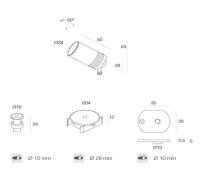
Model:Surface Mount PAR103A/B/C Wattage:3W Head rotary:360° Voltage:DC12V/AC110-240V Current:250mA LED Source:Osram LED CCT:2700-6000k Lumen:295lm CRI:Ra90 Beam angle:15/25/45° IP:IP20 Material:Aluminum Shell color:Anodised silver/black
