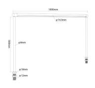
Model:Bridge 016 Wattage:16W/Meter Voltage:DC12V/DC24V PC cover:Milky/clear Length:Custom made Height:Custom made LED Source:Osram SMD CCT:2700-8000k Lumen:100lm/Wattage CRI:Ra80/93 Beam angle:90° IP:IP20 Rotary:360°
