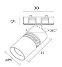
Model: Mini-Trak 101-2 Wattage:2W Head rotary:355° Voltage:DC12V/DC24V Non-dimmable LED Source:Osram LED CCT:2700-6000k Lumen:120-180lm CRI:Ra80/93 Beam angle:15/30/60° IP:IP20
