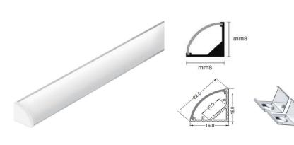
Model:Linear 2301 Size:16\*16mm/8\*8mm Length:200-2000mm Custom made Voltage:DC12V/DC24V LED Source:Osram LED CCT:2700-6000k Lumen:100lm/W CRI:Ra80/93 Beam angle:120° IP:IP20 Material:Aluminum Shell colour:Anodised silver/black
